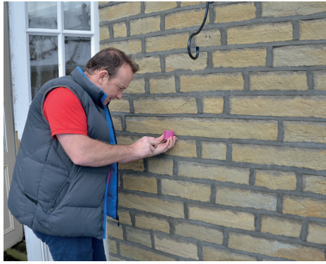
Exterior set-up of U-value testing sensor
