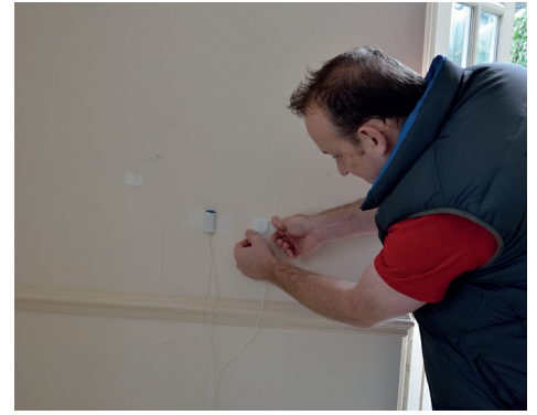
Pre-treatment set-up of U-value testing sensor
